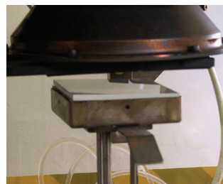
Ignited using a 10,000 V electric spark.
