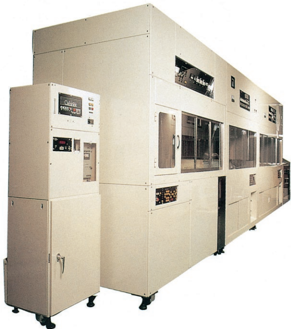
Fully automated wet wafer cleaning equipment (TND)
