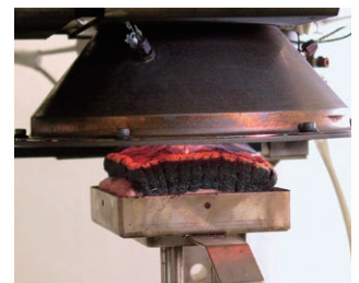
The material carbonizes without igniting.
