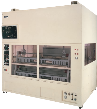
Automatic equipment for quartz tube cleaning (TSP, TS)
